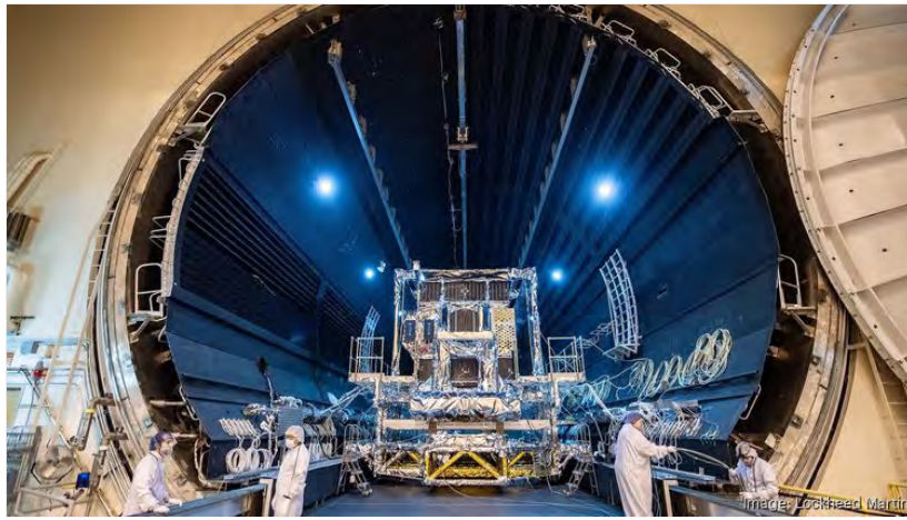
Workers at Lockheed Martin Space move a missile warning satellite, known as SBIRS GEO 5, into a thermal vacuum testing chamber in April 2020, in preparation for later launch.
