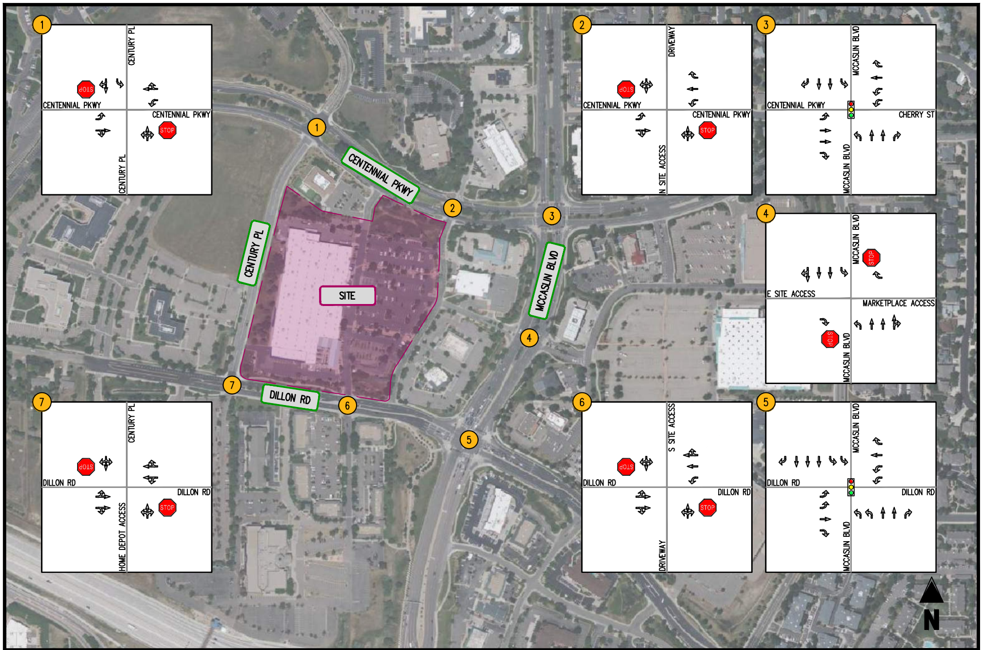
FIGURE 2-1 EXISTING LANE USE AND TRAFFIC CONTROL
