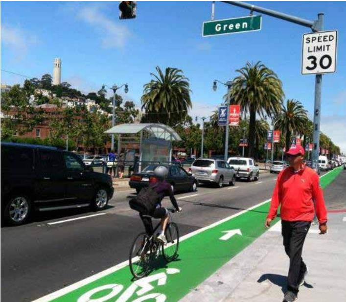
Complete Street with Separated Bike Lane
