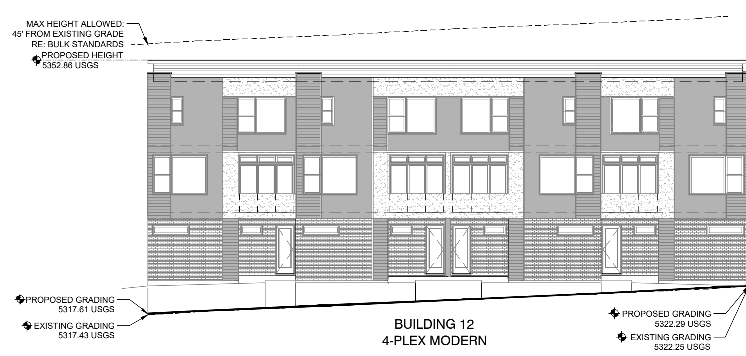
BUILDING 12 - NORTH ELEVATION 1/16" = 1'-0"
